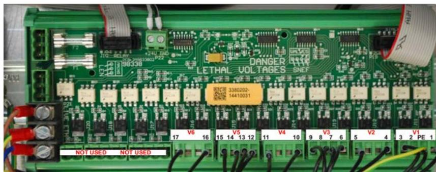
**Figure 23. Solenoid Valves Connection Guide**
