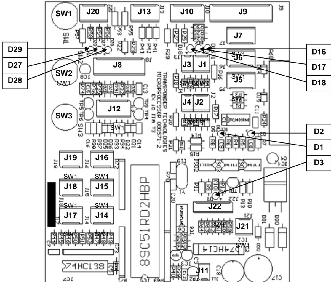
Figure 3 – Component Locations on 080563-4
