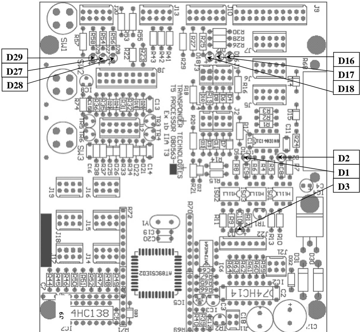
Figure 2 – Component Locations on 080563-5
