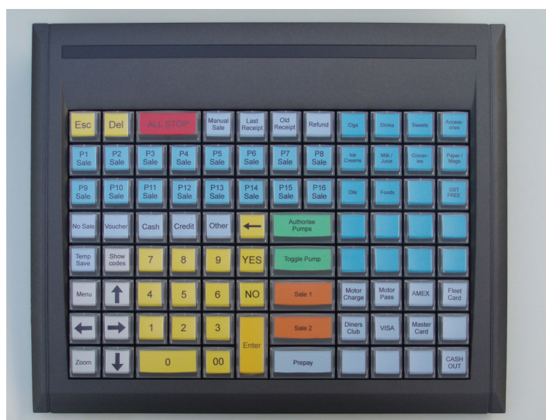
Figure 5-2: TT Keyboard (96-key, Type A – no card swipe reader fitted)
