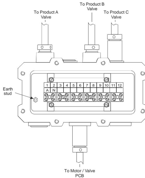
Figure 50 – Valves J-Box(s) Lowline Mk3 Pumps and Dispensers
