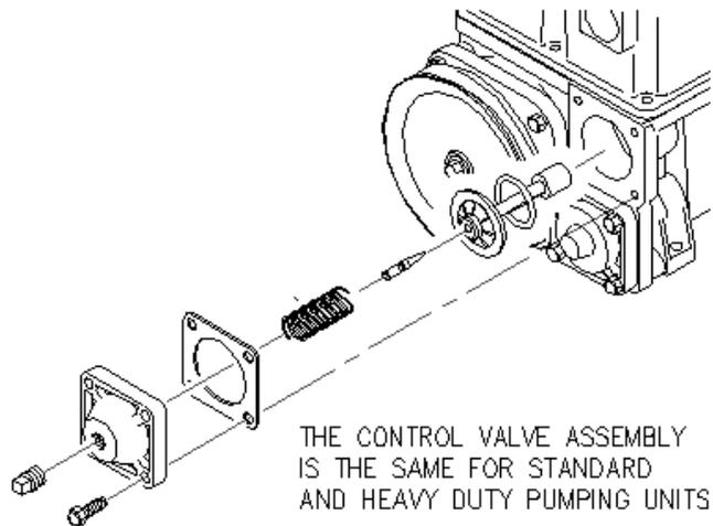
*Figure 41 – GPU-90 - Control Valve removal*
