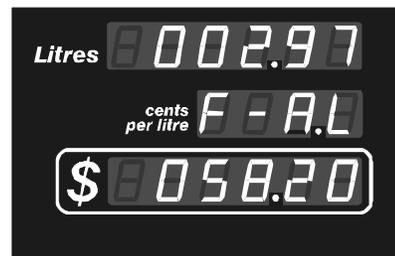
Figure 15 – Example of Front Hose "A" Volume Totals – i.e. 297,058.20 Litres
