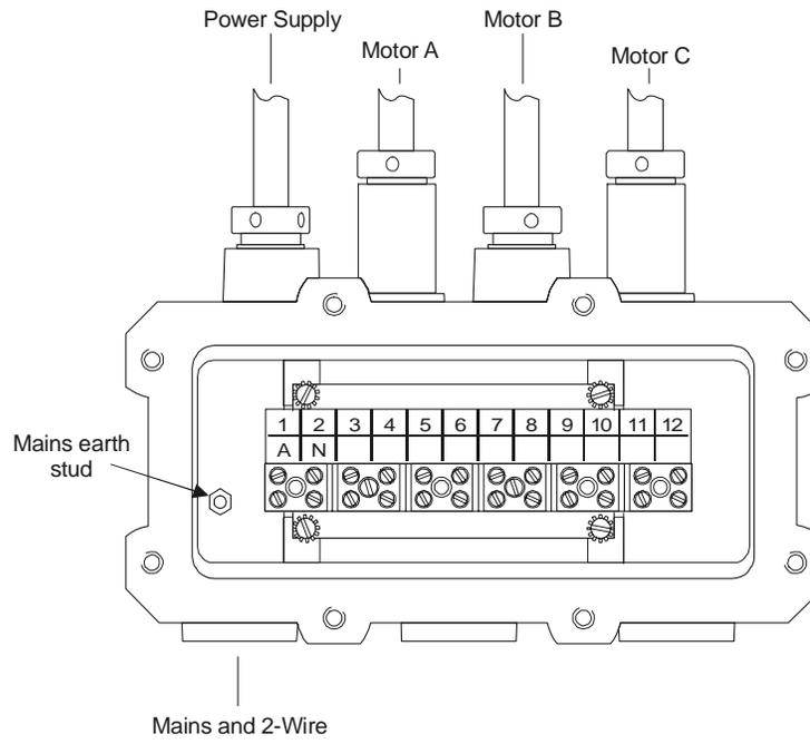
*Figure 49 – Mains J-Box for Lowline Mk3 Pumps*
