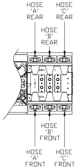
Figure 54 – Nozzle Switch Assignment Positions
