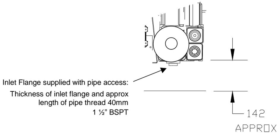
Figure 3 – Hydraulic coupling - Pumps
