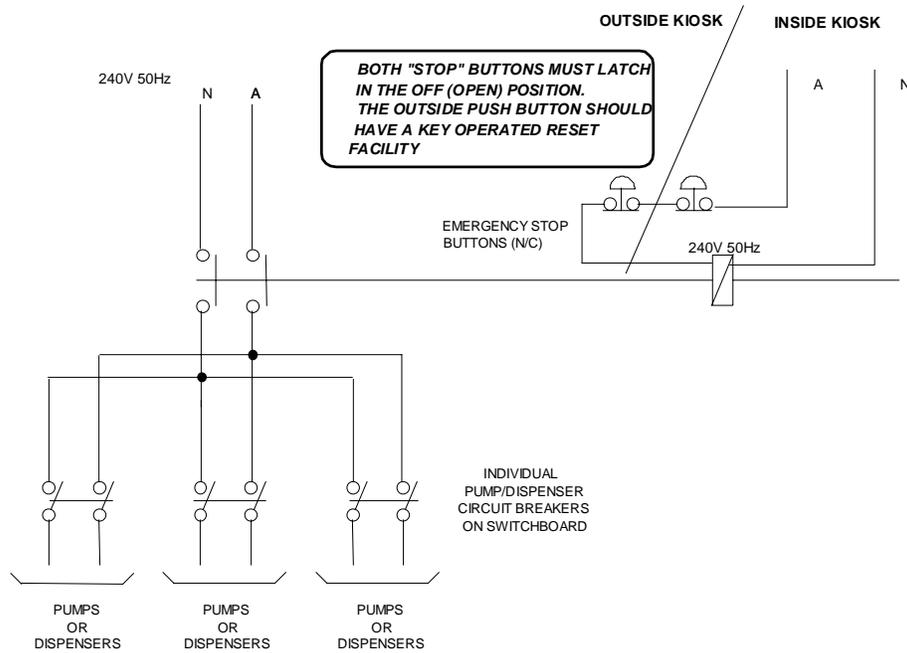
Figure 1 – Emergency Power Cut-off circuit
