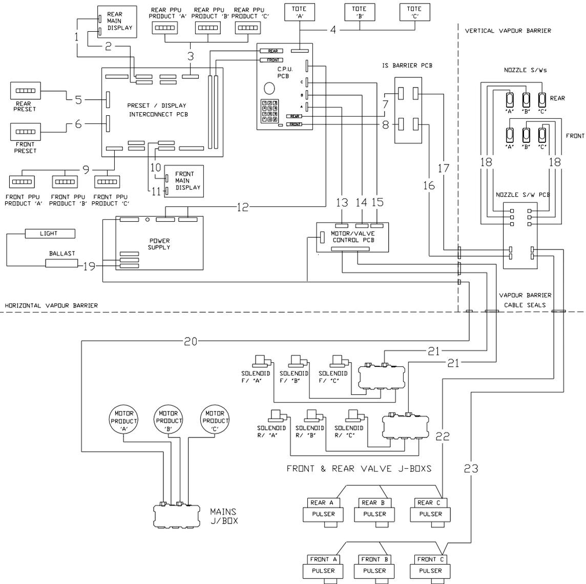
Figure 57 – Cabling Diagram – Six Hose Three Product Lowline MK3 Pump and Dispenser
