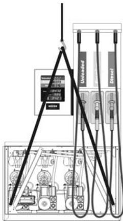
Figure 5 - Lifting Arrangement
