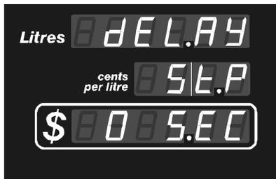
Figure 18 – STP Delay time in Seconds. Enter from 0 to 9.
