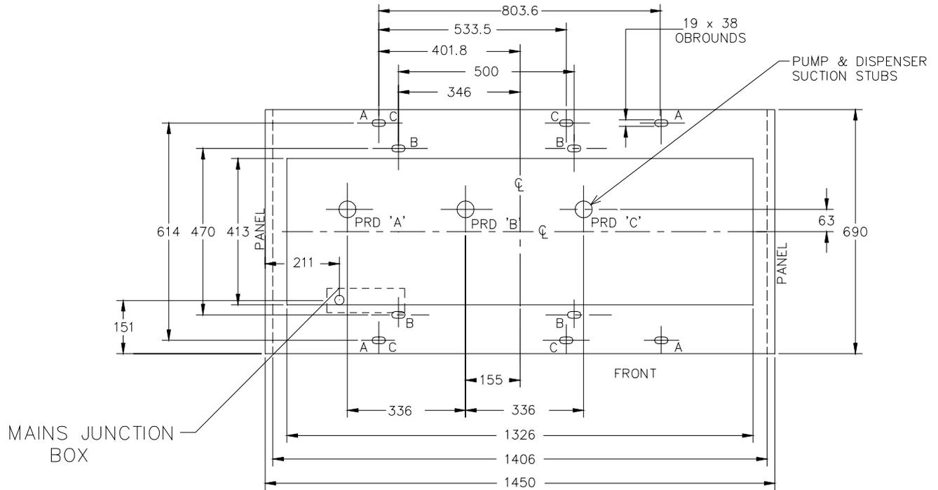
Figure 2 – Mounting footprint for Lowline MK3 Pumps and Dispensers
