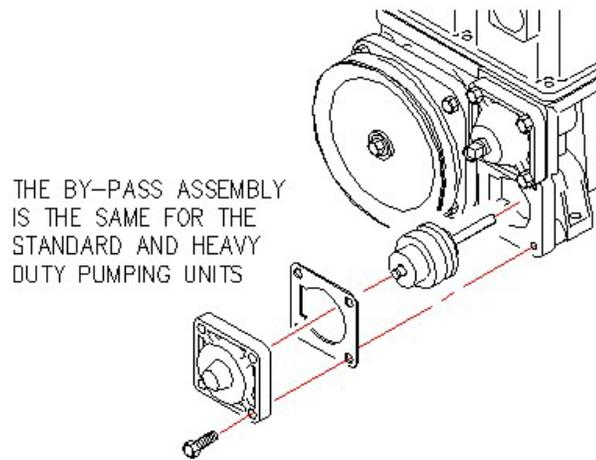
Figure 40 – GPU-90 – BY-Pass Pressure Valve removal
