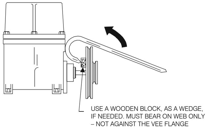
*Figure 42 – GPU-90 – Pump Pulley removal*
