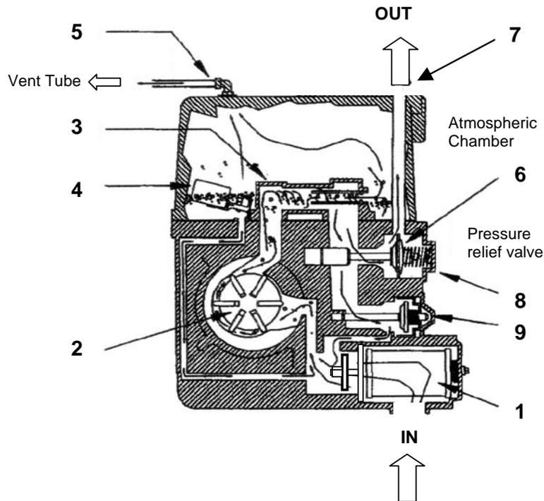
Figure 21 – GPU-90 Pump, Operation Diagram
