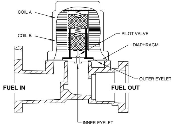
Figure 22 – Flow Control Valve
