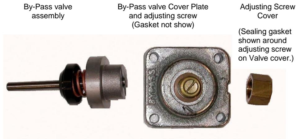
The pumping unit uses a bypass valve assembly in order to relieve the pumping unit pressure when the motor is running, but no fuel is being dispensed.
