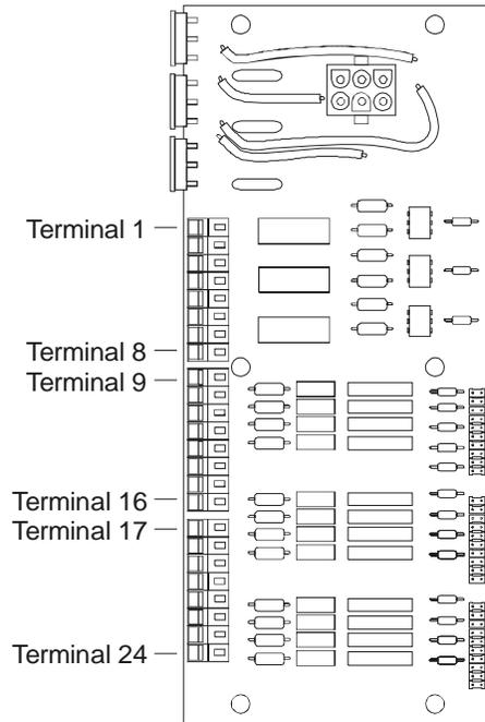
Figure 51 – Motor/Valve PCB – Layout.
