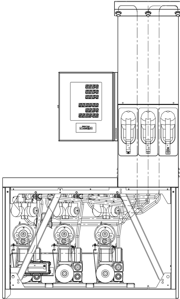
Figure 23 – Hydraulic Configuration – Six Hose Three Product Pump
