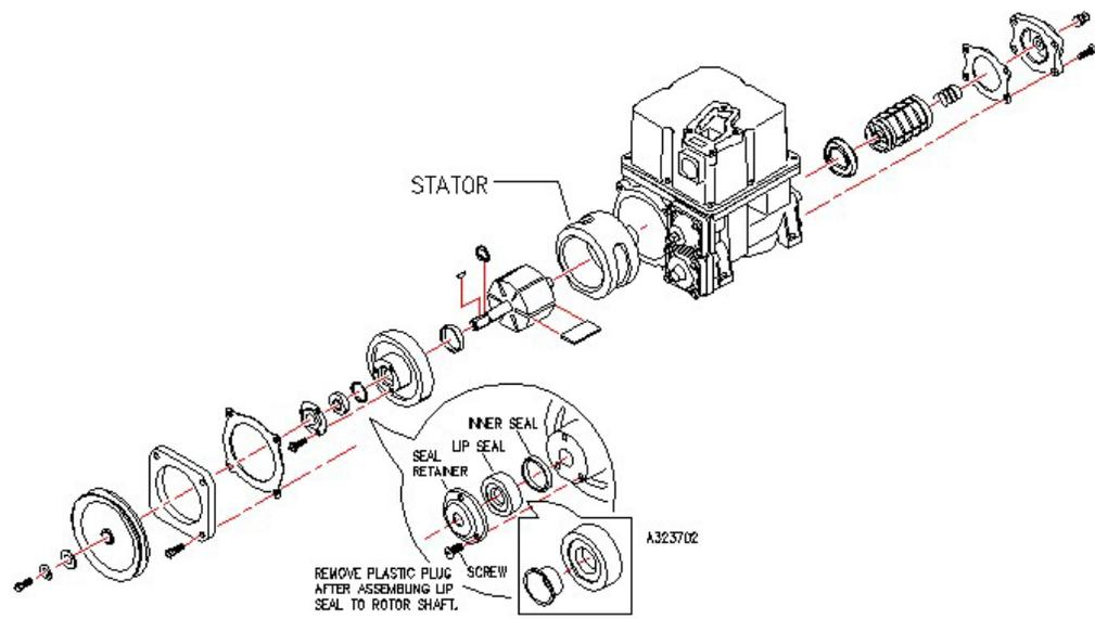
Figure 43 – GPU-90 – Pump cartridge and Inlet strainer assembly
