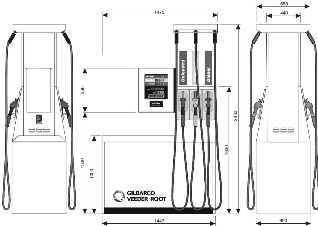
Figure 48 – Dimensional view – Six Hose- Pump or Dispenser
