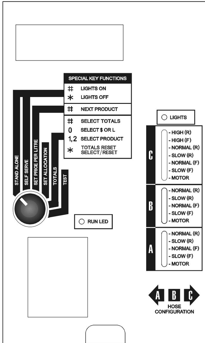
Figure 27 – Manager Function Panel – Lowline Mk3 Pump
