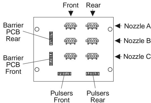
Figure 56 – Nozzle Switch I/F PCB – Cable plug positions
