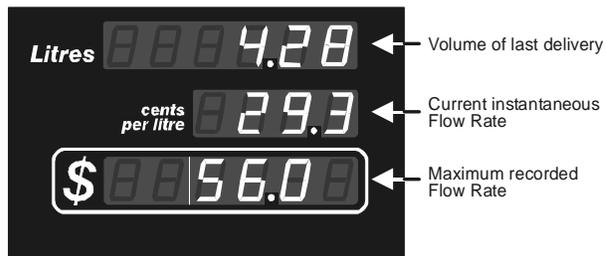
*Figure 37 – Flow Rate Test Display*
