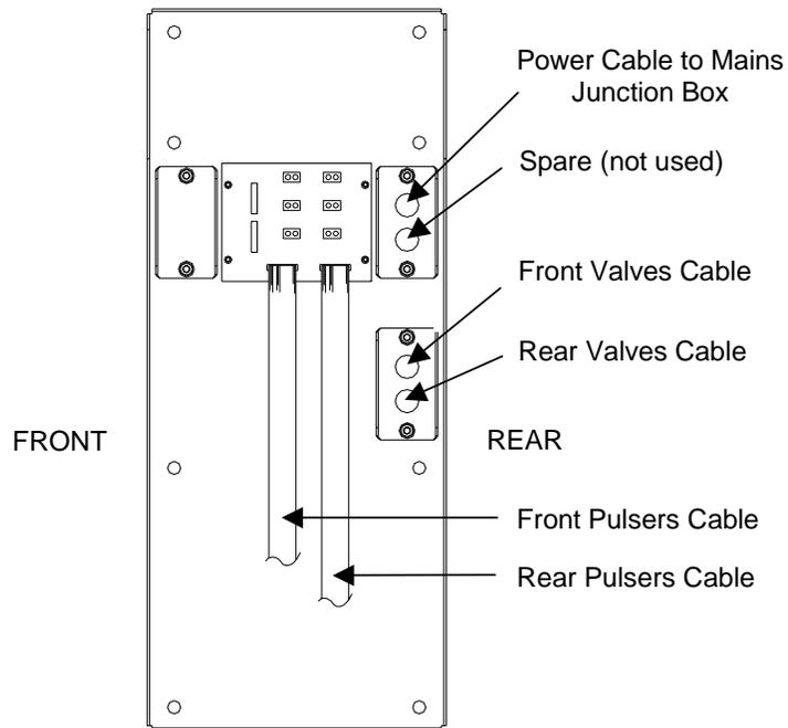
Figure 53 – Vapour Barrier Cable Position, CDM Vertical Barrier
