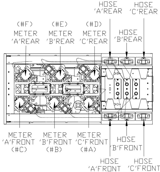
Plan View of 6 Hose – Hose to meter assignment
