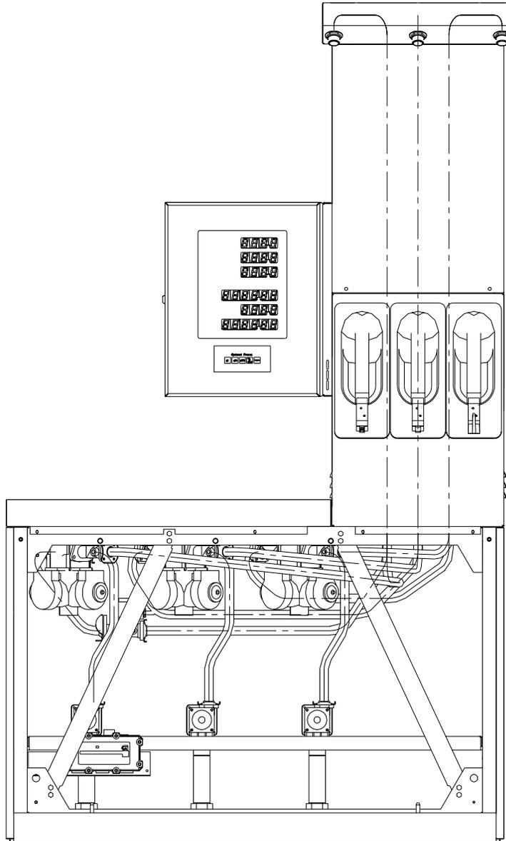
*Figure 24 – Hydraulic Configuration – Six Hose Three Product Dispenser*
