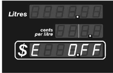
Figure 29 – Earthquake Sensor status
