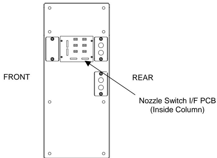
Figure 55 – Nozzle Switch I/F PCB – Column mounting position
