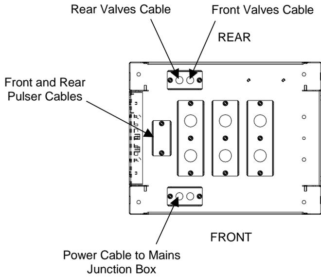
Figure 52 – Vapour Barrier Cable Position, Column Horizontal Barrier
