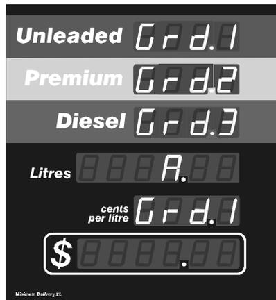
Figure 11 – Main and PPU Display digits with Grade Data
