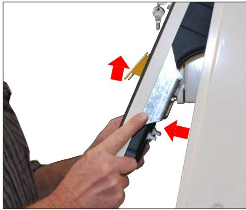
b Pull the holster panel out at the bottom and lift up to remove from the top panel.
