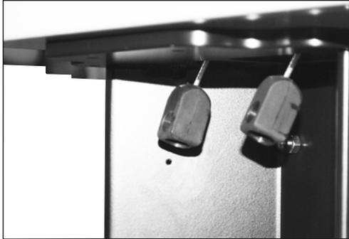
Anchor points underneath the C-Spreader
