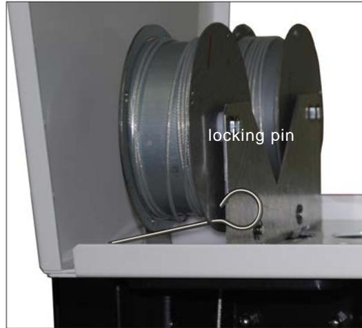
b While maintaining the tension on the reel, secure it by inserting the locking pin as shown above.
