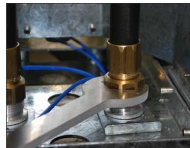
3. Secure the hose by fastening the 3-hole flange to the spreader base plate.
