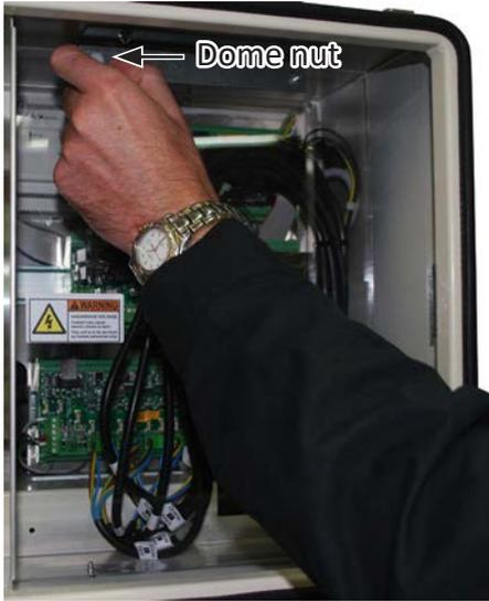
1. At the rear of the head remove the shield covering the gear plate by first removing the dome nuts on the top of the shield.
