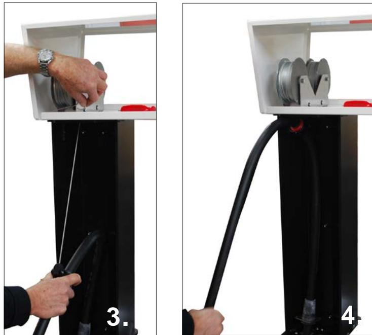
3. Maintain tension on the cable while pulling the hose down to remove the locking pin.
