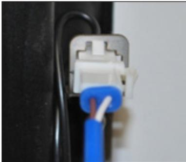
c Connect the holster switch cable. (See Section 6)
