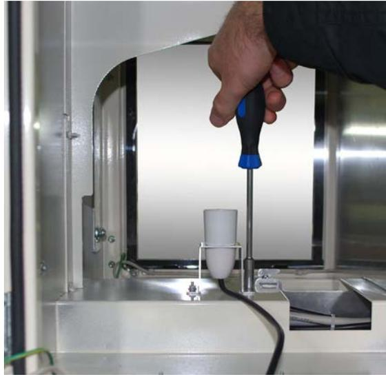
2. Fit the light mounting bracket to the 2 studs in the middle of the head. Secure with 2 M4 nuts.
