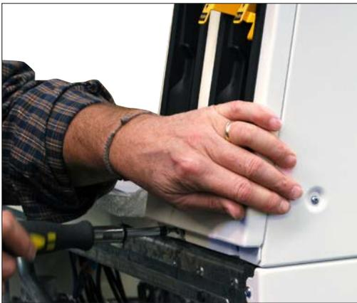
a Remove both screws at the bottom of the holster panel.
