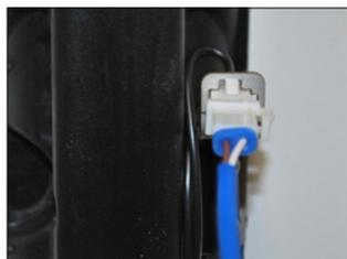
c Disconnect the holster switch cable. (See Section 6)
