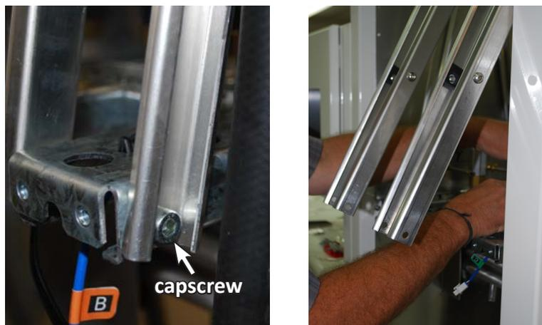
**Figure 30. Gaining Access by Moving the Channel Runners**
