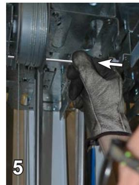
When locked the wire loop should be approx. 20-30mm above the hose carriage (5).
