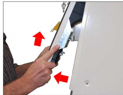
(b) Pull the holster panel out at the bottom and lift up to remove from the top panel.
