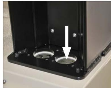
2. Fasten the brass end of the hose to the column.
