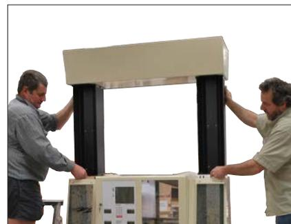
(b) Carefully lower the base of the spreader unit down on the top of the dispenser.
