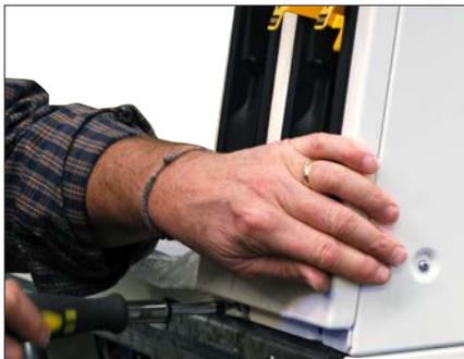
(a) Remove the 2 screws at the bottom of the holster panel.
