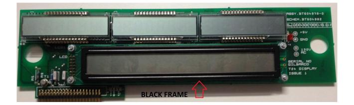
The Display will not function if placed in a T24 Console POS Unit containing an early Main Processor PCB that has not been through Kentronics or Gilbarco for the appropriate upgrade.
