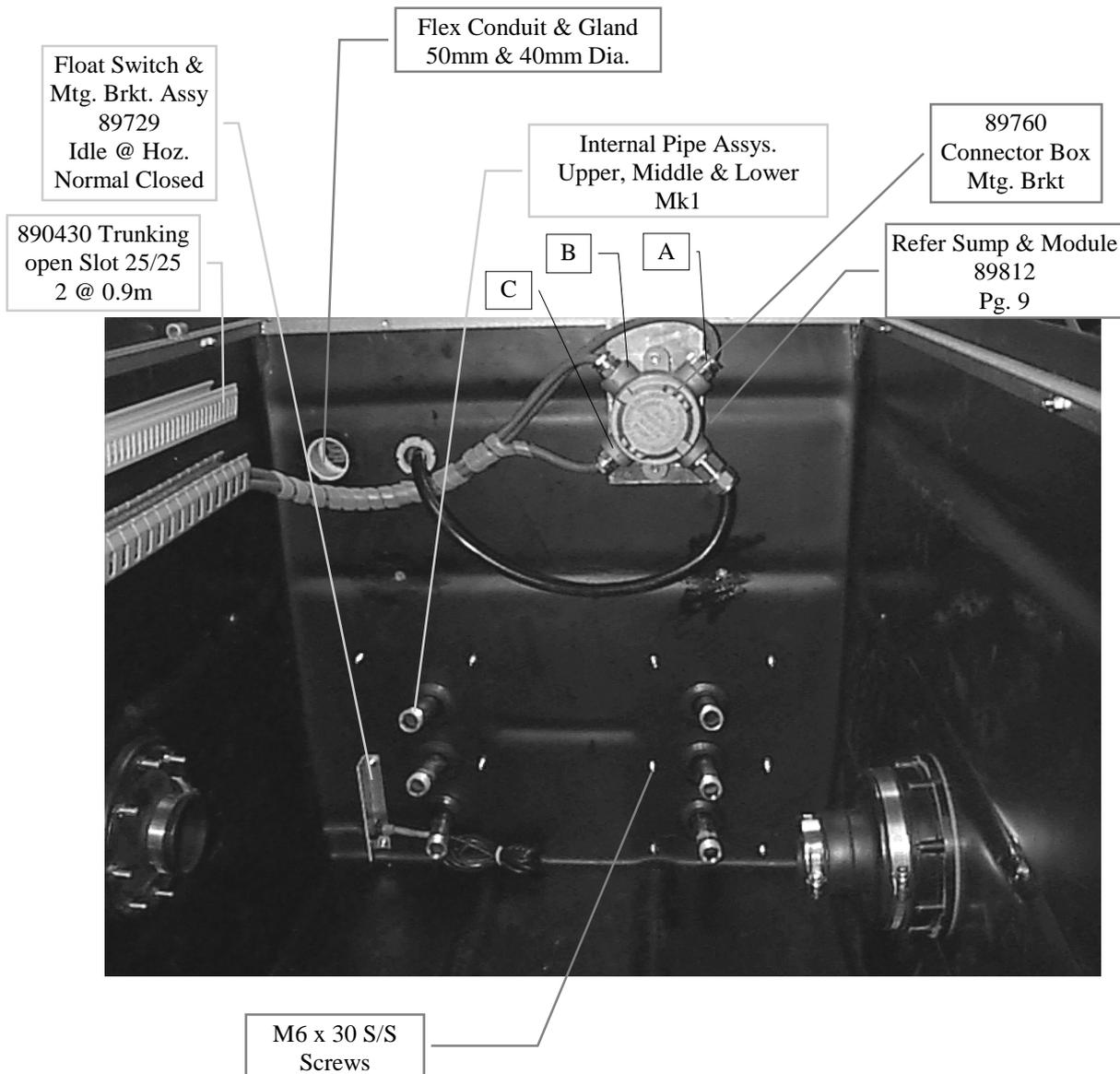
Bulkhead Seals for Product Feed line & Internal Delivery Pipes are fitted at PEC as part of original Sump
