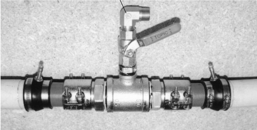
Note distance between test point seals on assy. shown above must be min possible .
