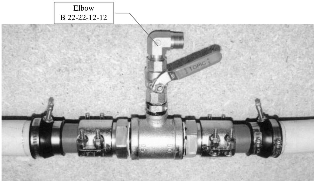
Note distance between test point seals on assy. shown above must be min possible .
