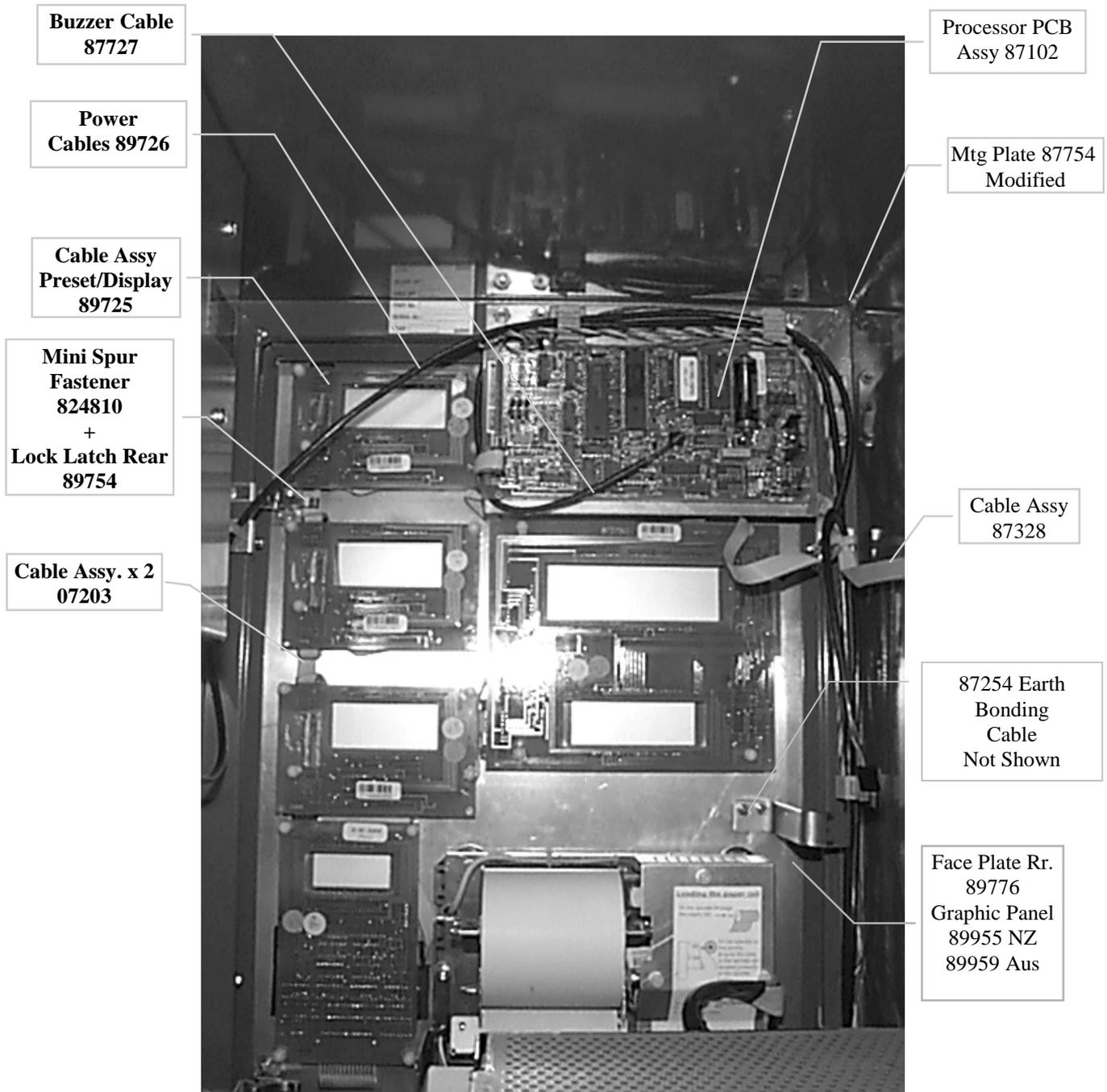
**Display & Preset PCB's as per Front Door Assy Pg 6**
