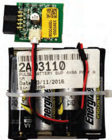
Figure 110. PULSE Battery BUP 4xAA Pack Assembly
