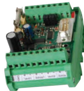
Figure 117. VR2 Bürkert 1094EV Controller
